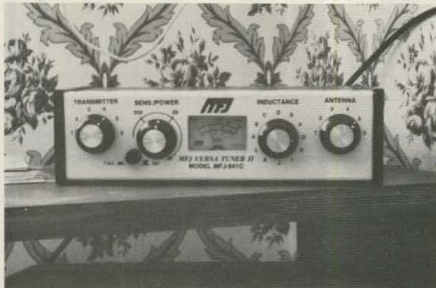
Swr meter showing the swr (the tuner was bypassed).
